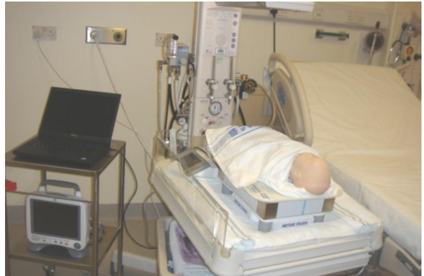
Figure 2: Set up of scales on resuscitaire next to delivery room bed, doll demonstrating closeness to mother during weighing.
